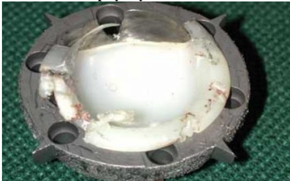
Plate 9: Shows severe wear and fracture of the polyethylene liner
